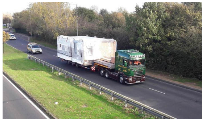
The first Swan home being delivered to site.
